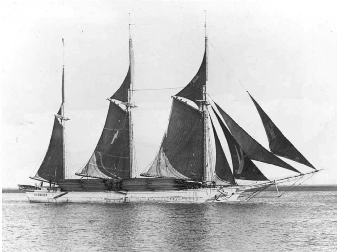
Figure 2. The Kate Gillett after her 1882 rig change from two to three masts, and name change to Horace H. Badger . Historical Collections of the Great Lakes, Bowling Green State University.
