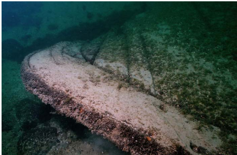
Figure 19. Foot of the starboard bow, showing the stempost, stem iron, and iron reinforcement strap. Photo by Tamara Thomsen.
