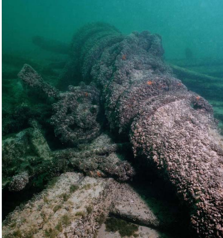
Figure 17. Kate Kelly 's windlass with pinion gear and hand lever. Photo by Tamara Thomsen.
