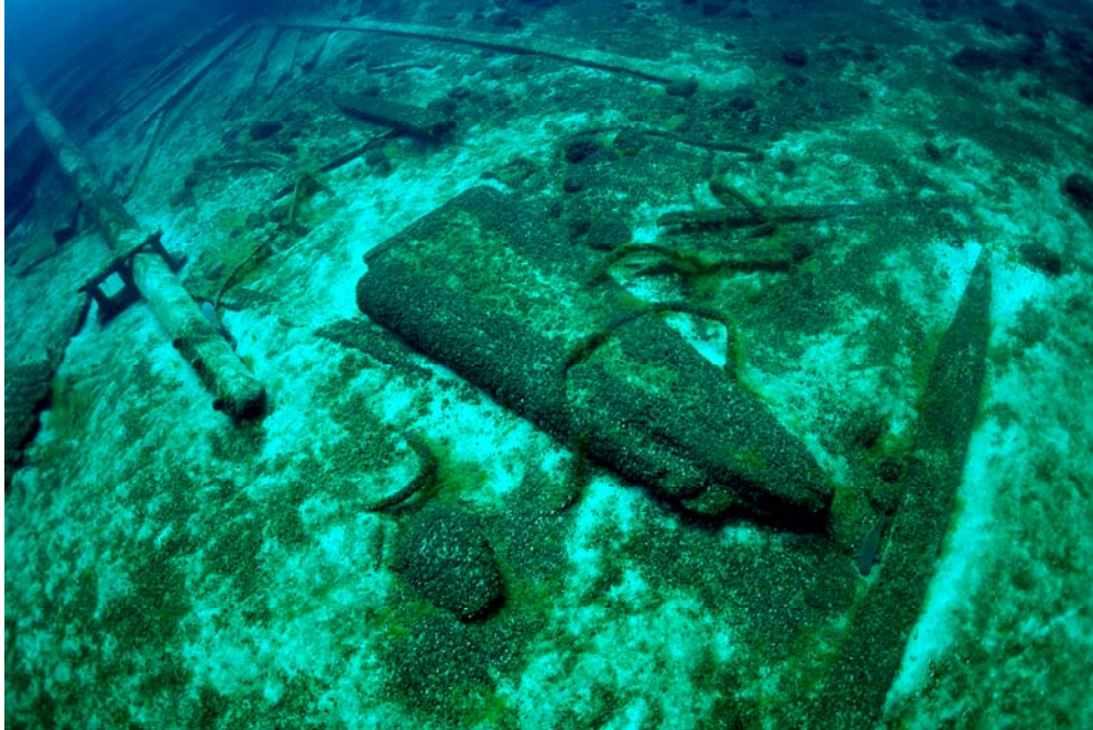
Figure 13. The Daniel Lyons ' rudder. The mizzen masthead and trestle tree are visible to the left. Photo by Tamara Thomsen.
