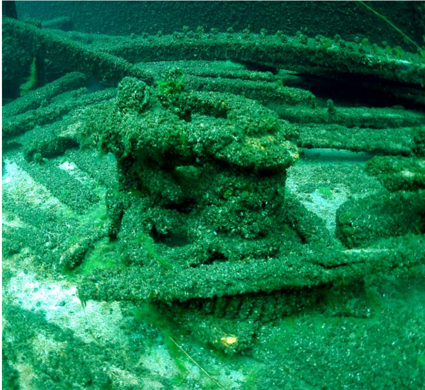
Figure 11. Centerboard winch. Photo by Tamara Thomsen.
